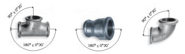
During assembling of fittings the deviations  $+/-0^{\circ}30'$  cause the deviations of the pipelines from the axis (both in the horizontal plane as well as vertical plane). In case of long, multisegment pipelines, the deviations may be summed.
